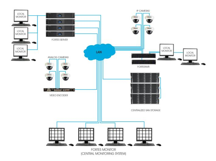
NOTE. The above network configuration is a conceptual overview only and is not intended to show a detailed network topology. The actual network requirements for your installation will differ based on the configuration, requiring changes or perhaps additional network equipment. Please contact Infinique representative to discuss your specific requirements.
